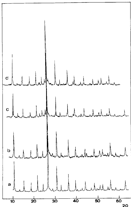
Fig. 10. X-ray diffraction patterns of K_3PMo_{12}O_{40} calcined at 500^\circ C (a), K_3P_1Mo_{11}Sb_1Fe_1Cr_{0.5}Ce_{0.25}O_n spent after 50 h time-on-stream (b), K_2P_{1.2}Mo_{10}W_1Sb_1Fe_1Cr_{0.5}Ce_{0.75}O_n calcined at 500^\circ C (c) and spent after 100 h time-on-stream (d).
